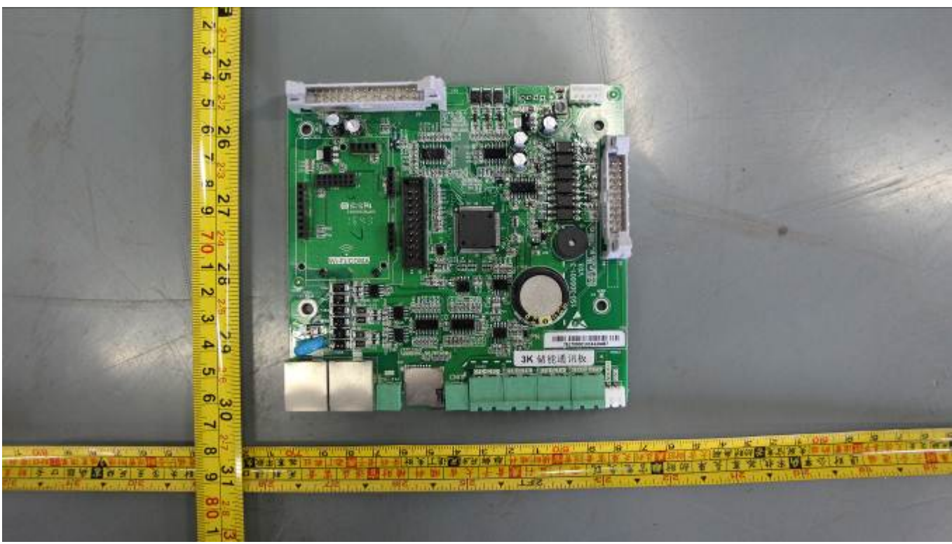
Communication board view
